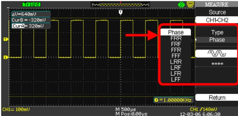
First select a **Source Channel** for your **Delay** measurement parameter by pressing the Source option button. Now, use the **Type** option button to choose from the following Delay measurement parameters for your selected source.
