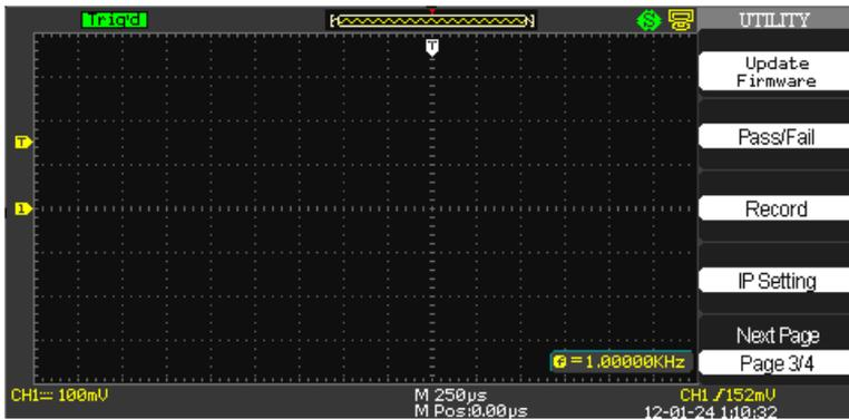
1. Press the **Update Firmware** option button to update the oscilloscope using the USB memory device. For more information, see the **Updating the System Software** (on page 80) section.
