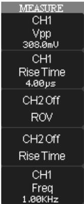
Access parameter measurements by pressing the **MEASURE** front panel button. The main Measure menu is shown. Notice how each row on the Measure menu is labeled with a **CHX**, a **Type**, and a **Value**. Each row is a customizable parameter measurement preset.
