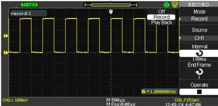
1. Press the **Source** option button to choose from CH1 and CH2 (also, CH3 and CH4 on four channel versions) as the recorded signal input.
