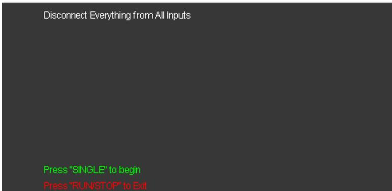
2. As the screen indicates, disconnect anything plugged into input connectors (except for the power cable) before pressing the **SINGLE Front Panel** (on page 7) button and performing a self-calibration. Press the **RUN/STOP** front panel button to exit the **Do Self Cal** screen.
