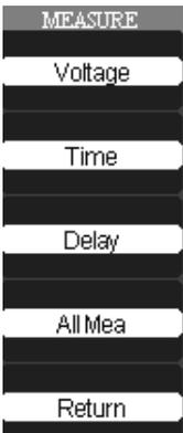
Press the corresponding option button to show additional preset controls for **Voltage**, **Time**, **Delay**, and **AllMea** for the Source channel selected.
