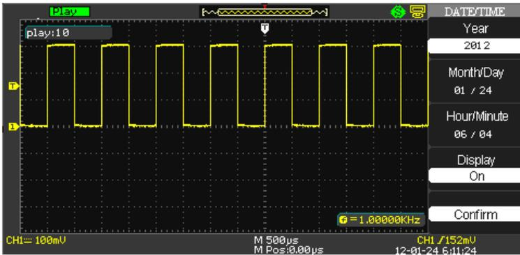
1. Press the **Year** option button and use the Adjust **Front Panel** (on page 7) knob to provide a year value.
