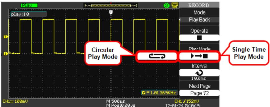
3. Press the **Interval** option button and use the **Adjust** front panel knob to dial in the desired interval between record frames for the playback of your recorded waveforms.
