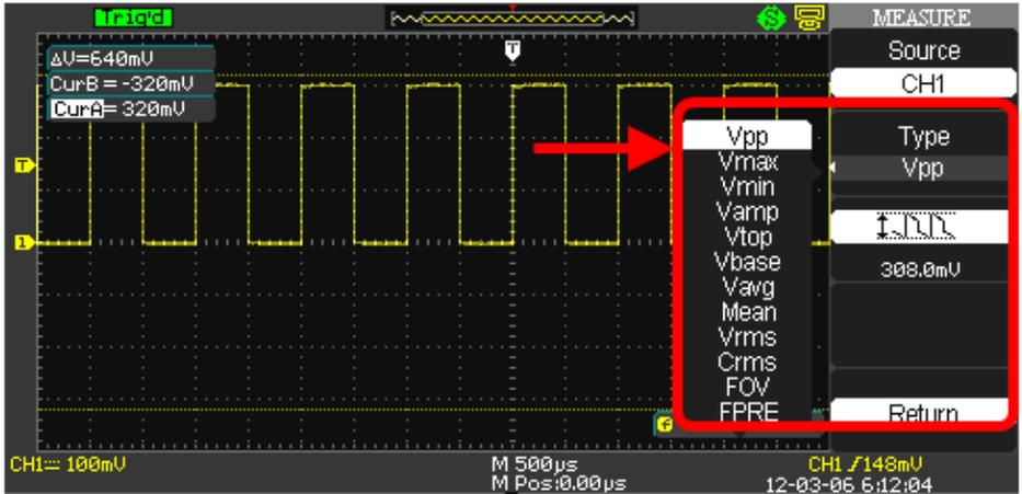
First select a **Source Channel** for your **Voltage** measurement parameter by pressing the Source option button. Now, use the **Type** option button to choose from the following Voltage measurement parameters for your selected source.
