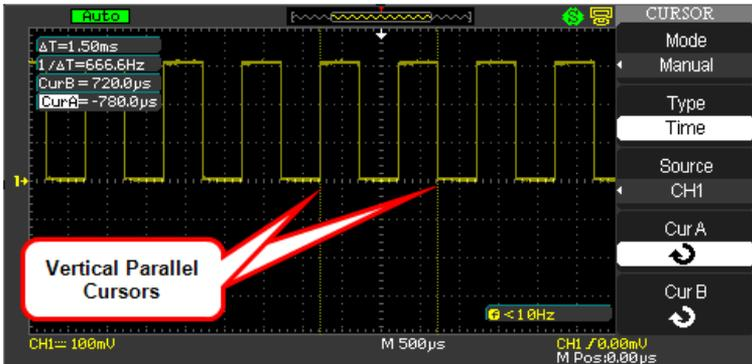
Move cursors by pressing corresponding **CurA**, **CurB** option buttons, and then using the **Adjust** front panel knob. Before using cursors, you should make sure that you have set the signal source as the channel for measuring.
