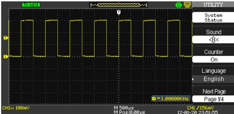
1. Press the **System Status** option button to display a summary of the oscilloscope settings.
