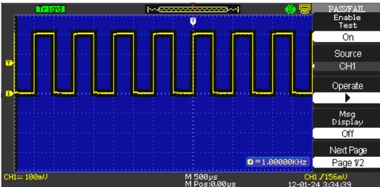
**NOTE:** Turning **Enable Test On/Off** allows you to control whether or not the mask is shown on the display grid area while making your settings. The **Operate** button runs the test and allows you to see the results update in real time.
