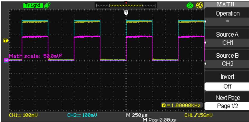
2. The **Source** can be any channel, but not another math trace. Channel behavior for the math operators allow for **CH1-CH2** or **CH2-CH1** selections.
