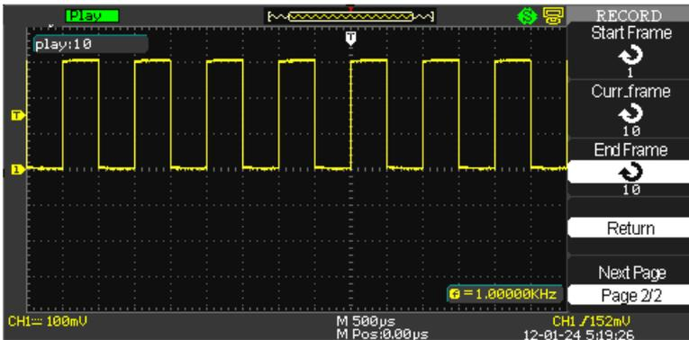
1. After pressing **Next Page** from Page 1/2, press the **Start Frame** option button and use the **Adjust** front panel knob to dial in the specific frame of your recorded waveforms where you want to start the playback.
