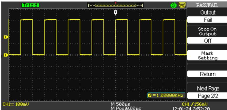
1. Press the **Output** option button to either **Pass** or **Fail**.
