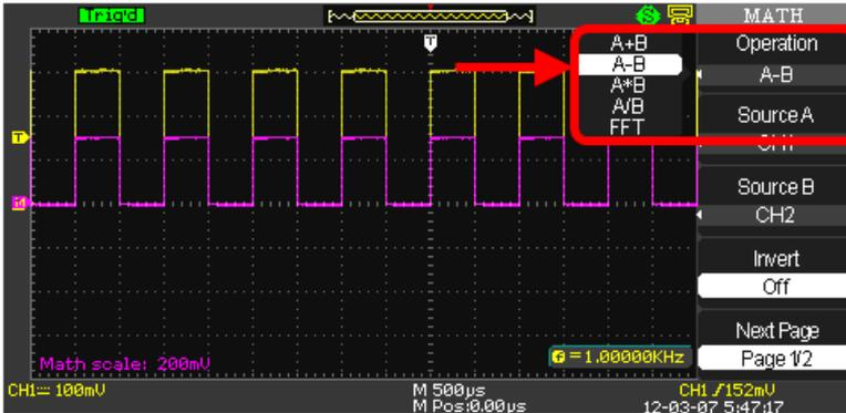
2. The **Source** can be any channel, but not another math trace. Channel behavior for the math operators force **CH1+CH2** or **CH3+CH4** selection pairings (using addition as an example).
