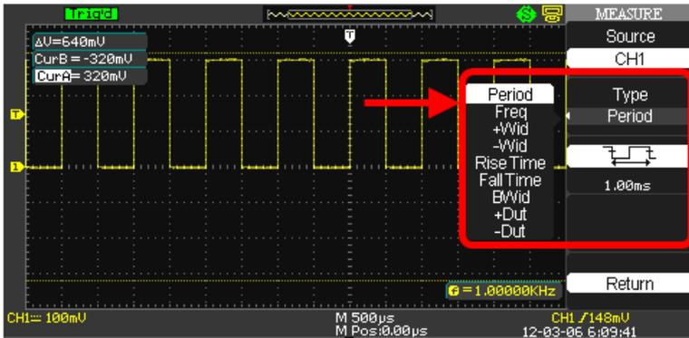
First select a **Source Channel** for your **Time** measurement parameter by pressing the Source option button. Now, use the **Type** option button to choose from the following Time measurement parameters for your selected source.
