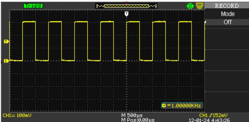
The **Record** function operates in three **Modes**: **Off**, **Record**, and **Playback**. As shown previous, no option button controls are available when the Record's **Mode** is set to **Off**.
