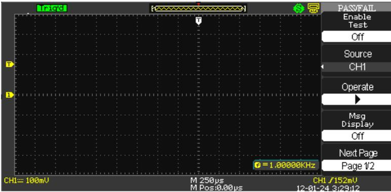
1. Press the **Enable Test** option button to turn the function **On** or **Off**.
