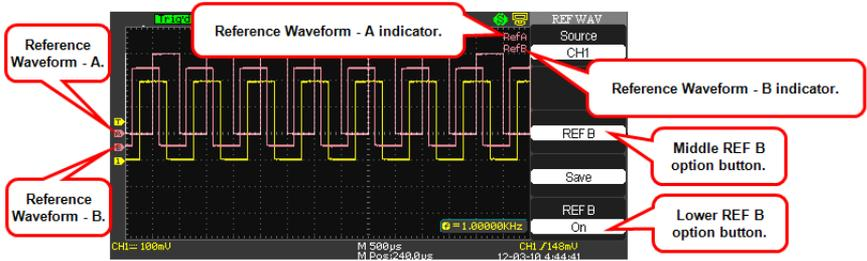
5. Use the **Save** option button to save your reference waveform for comparative analysis at a later time.
