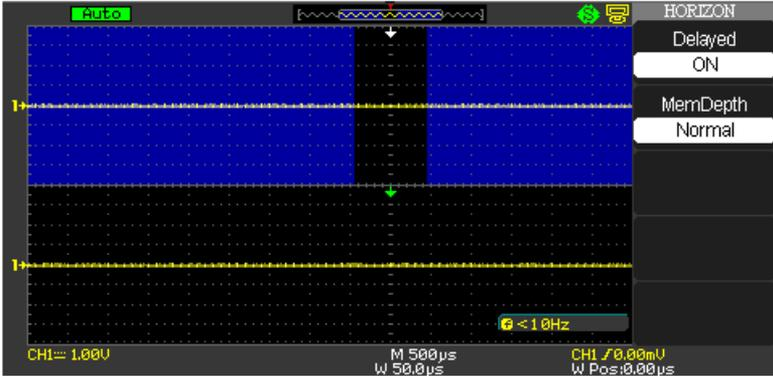
2. Press the **Delayed** option button on the **Horizontal** menu (or pressing the **Time/Div Front Panel** (on page 7) knob).
