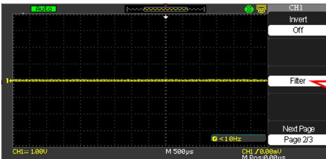
4. Press the **Filter** option button and select **On**.
