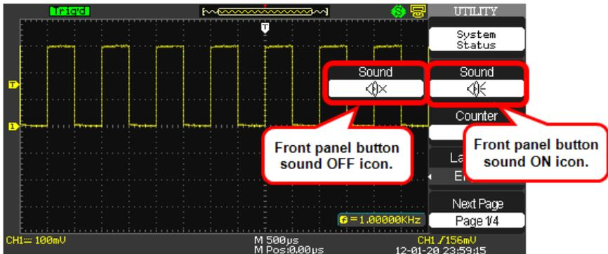
3. Turning the Frequency **Counter** On/Off shows or hides it from the grid display.
