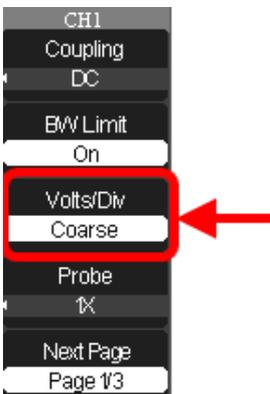
2. Now, press the **Volts/Div** option button on page 1/3 of the channel menu, and then select **Coarse (fixed)** or **Fine (variable)**.
