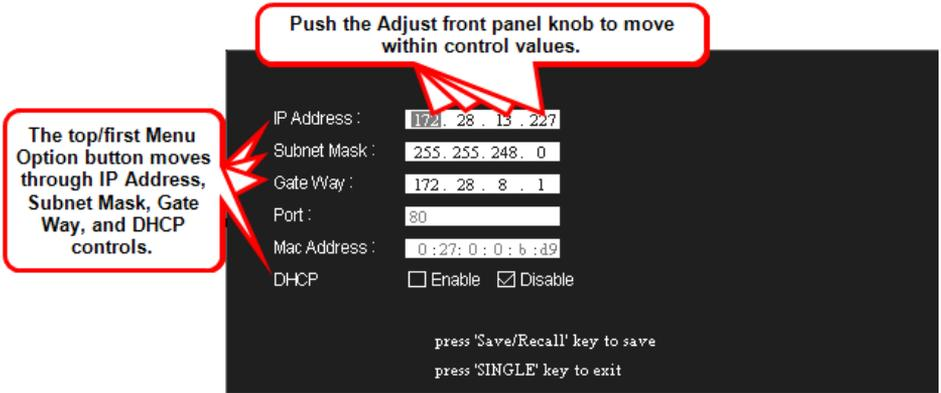
Use the top/first Menu Option button to move through **IP Address**, **Subnet Mask**, **Gate Way**, and **DHCP** controls. Push the **Adjust Front Panel** (on page 7) knob to move within a control and turn the knob to change values.
