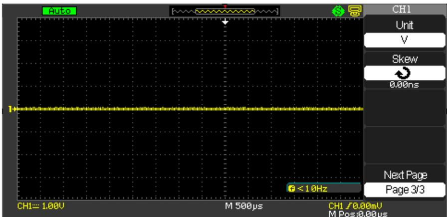
1. Pressing the Unit option button selects between **V** (Volts) and **A** (Amperes) values.
