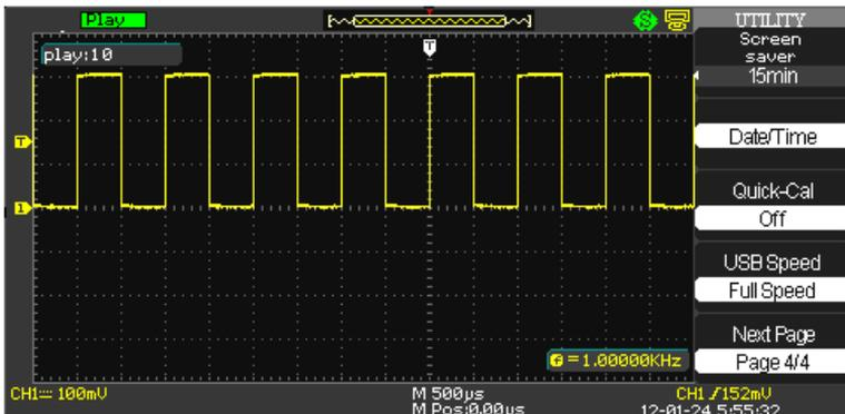
1. Press the **Screen saver** option button to choose from various time lengths before the oscilloscope display goes blank and enters screen saver mode. Time length options include **1min** , **2min**, **5min**, **10min**, **15min**, **30min**, **1hour**, **2hour**, **5hour** and **Off**. Of course, selecting **Off** keeps the oscilloscope from entering screen saver mode entirely.
