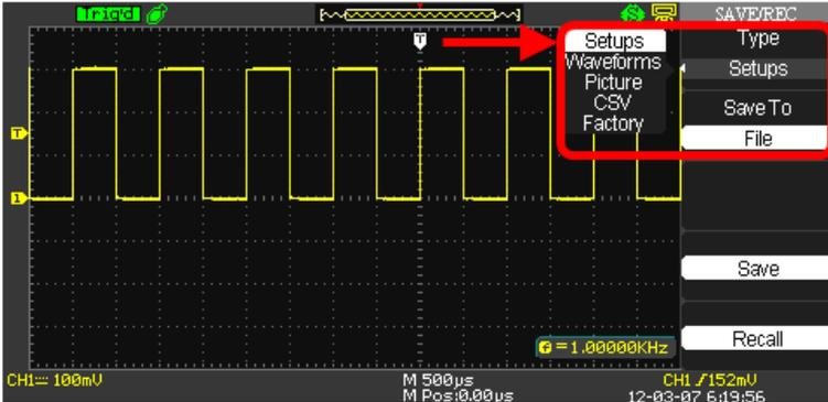
3. Save your setup either to **Device** (meaning internal memory on your WaveAce) or **File** (for storage on a USB memory device) using the following methods.
