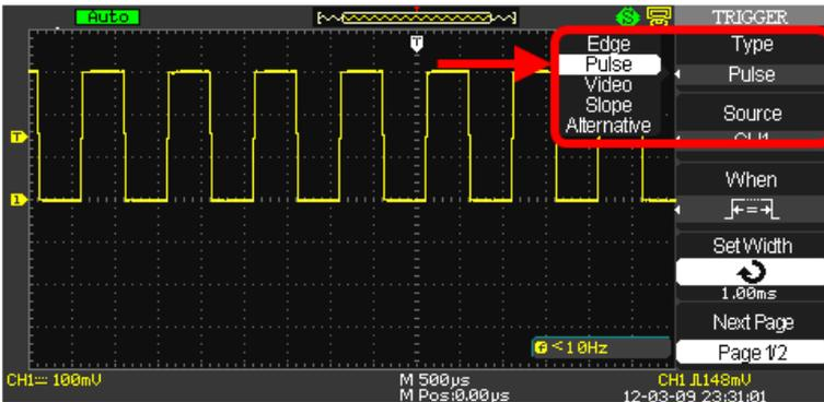
2. Press the **Source** option button to choose a channel input (**CHS 1 - 2**; or **CHS 1 - 4** on 4 channel models) or **EXT**, **EXT/5**, **AC Line** input.
