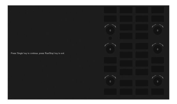
Press the "Single" button and the first LED on the front panel will light. The corresponding position of the key on the screen will also change color. Press the "Single" button to check the next button. Press the "Single" button consecutively until all the backlights are tested.
