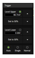
The lower level should always be less than or equal to the upper level. In the trigger descriptor box, the lower level is displayed.
