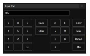
Let's use the operation of setting the "deskew" of a channel as an example: If the expected value is 65 ns, input "65" on the virtual keypad, and then choose the unit n to complete the operation. On the virtual keypad, touching the button Max, Min, and Default quickly set the parameter to its maximum, minimum and default values.
