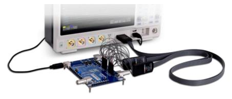
To connect the logic probe: Insert the probe, with the correct side facing up, until you hear a "click".
