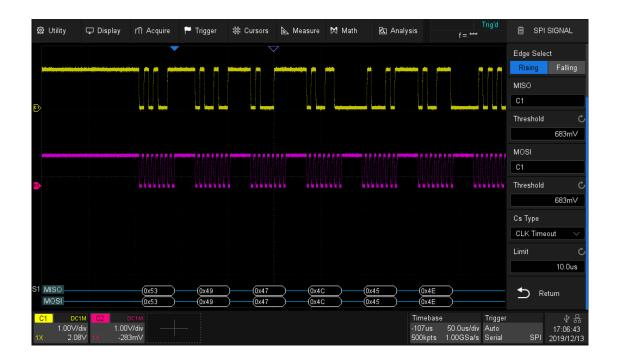
If the data width is set to be greater than 8-bits (such as 16-bits), measure the clock idle time between 8-bit data packets as 20  $\mu$ s, and then set the timeout time to a value between 20 and 300  $\mu$ s. In this example, it is set to 30  $\mu$ s:
