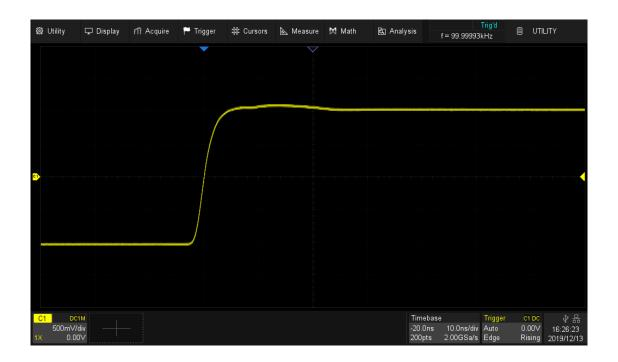
Timebase = 10 ns/div, Horizontal Delay = -20 ns = -2 div
