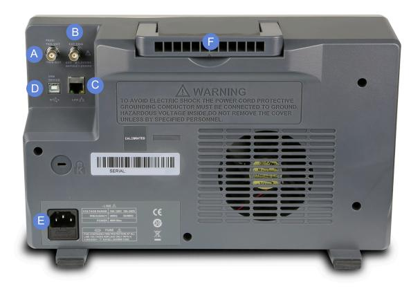
A. Auxiliary Out: Outputs the trigger indicator. When Pass / Fail is enabled, outputs the pass / fail signal.
