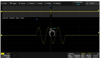
Adjust the horizontal position of the zoom area by dragging left and right in the zoom area of the main window or waveform in Zoom window
