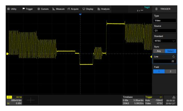
Trigger on a Specific Line of Video(NTSC)
