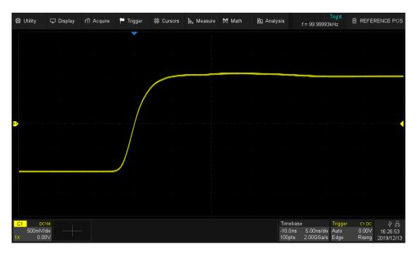
Fixed position, timebase is changed to 5 ns/div, the grid number of delay (-2 div) remains fixed, while the horizontal delay changes to -10 ns
