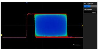
Segmented memory collection will store the waveform into multiple memory segments (up to 100,000) and each segment will store a triggered waveform as well the dead time information. The interval between segments can be as small as 2  $\mu$ s. All of the segments can be played back using the History function
