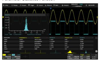
Statistics shows the current value, maximum value, minimum value, standard deviation and mean value of up to 12 parameters simultaneously. Histogram is available to show the probability distribution of a parameter. Trend is available to show the parameter value vs. time
