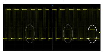
With a waveform update rate of up to 110,000 wfm/s, the oscilloscope can easily capture unusual or low-probability events. In Sequence mode the waveform capture rate can reach 500,000 wfm/s
