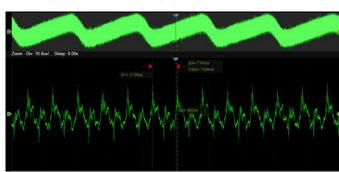
Using hardware-based Zoom technique and record length of up to 250 Mpts, users can select a slower timebase without compromising the sample rate, and then quickly zoom in to focus on the area of interest
