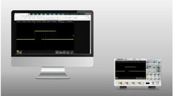
With the embedded web server, users can control the oscilloscope from a simple web page. This provides wonderful remote troubleshooting and monitoring capabilities
