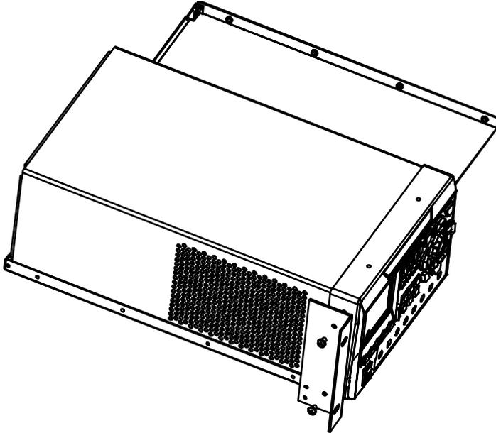
4. Fix the front filler panel to the right side of the front panel of the instrument using two M4 screws.
