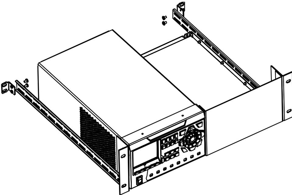
9. Install the rack mounted with the instrument into a standard 19 inch machine cabinet using eight M6 screws and eight M6 nuts.
