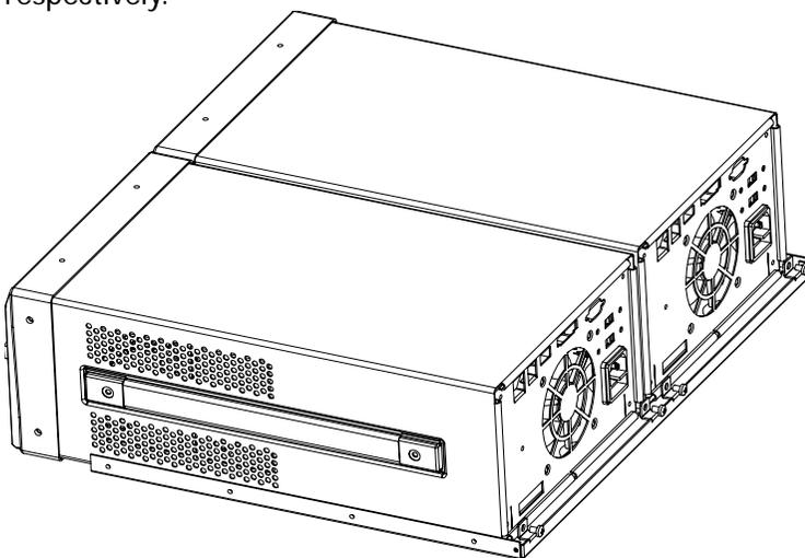
3. Fix the left fixing part at the left side of the front panel of instrument A using two M4 screws.
