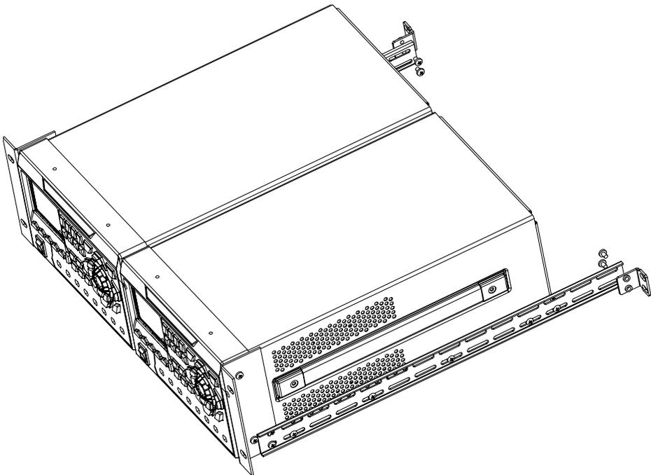
8. Install the rack mounted with the instruments into a standard 19 inch machine cabinet using eight M6 screws and eight M6 nuts.
