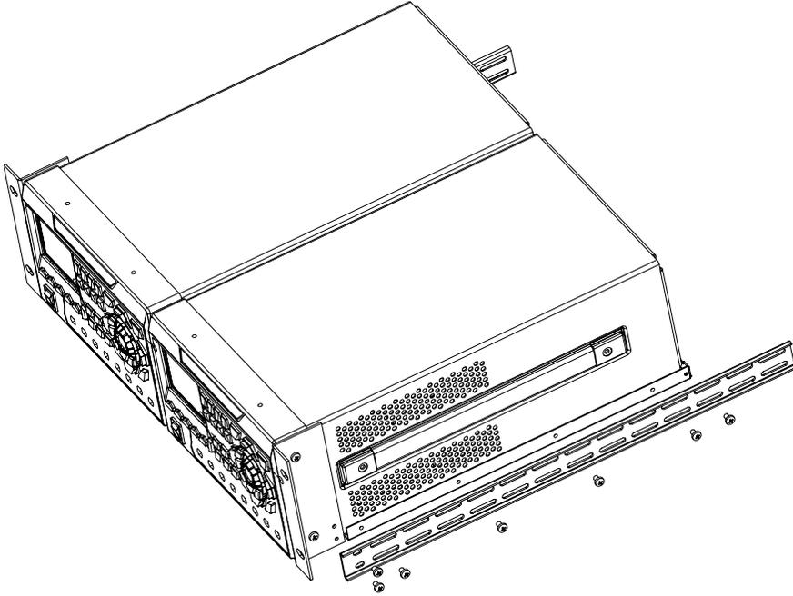
7. Fix the two side beam fixing parts to the end parts of the left and right rack rails respectively using four M4 screws.
