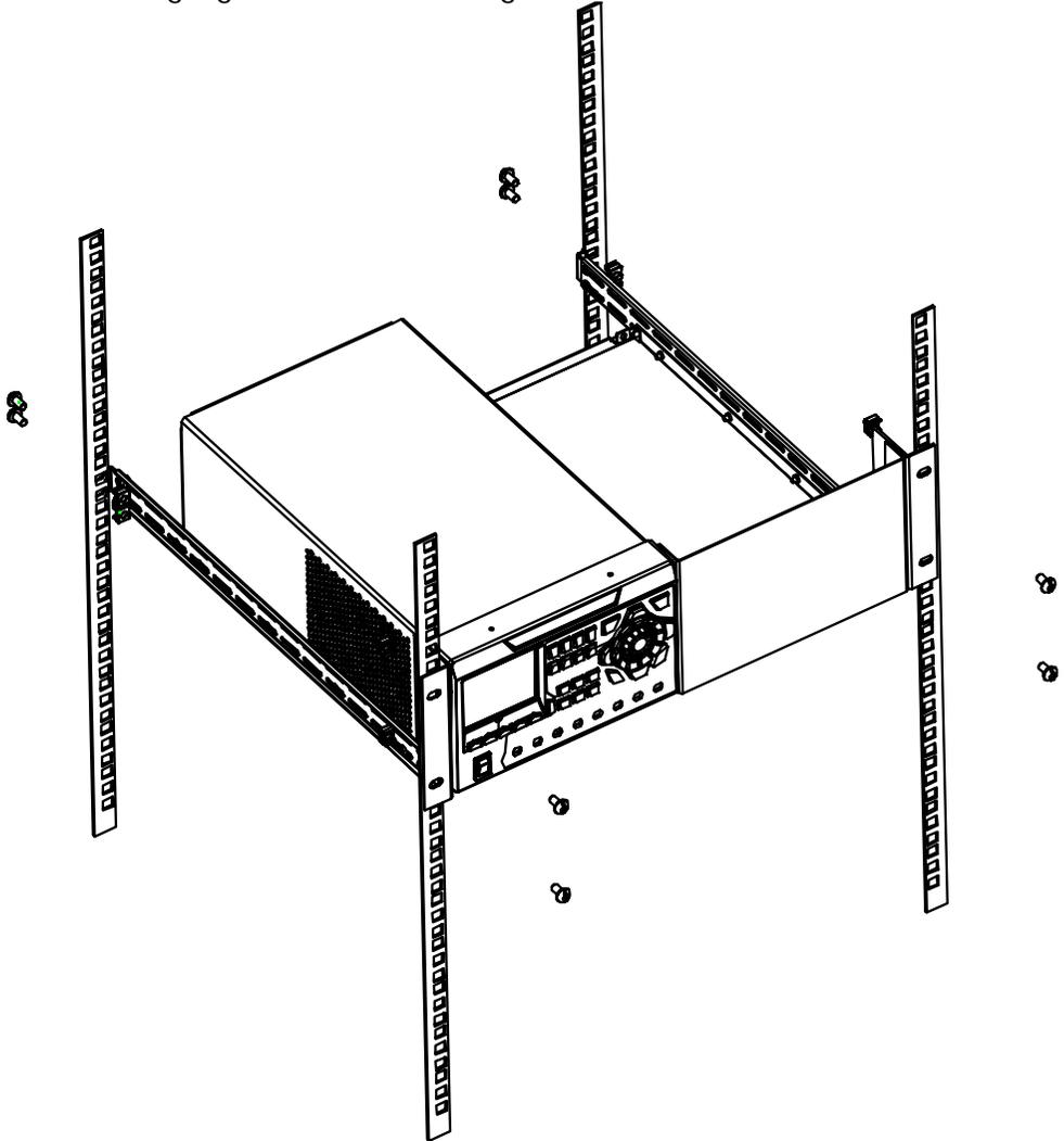
10. At this point, the diagram of the instrument is as shown in the figure below.
