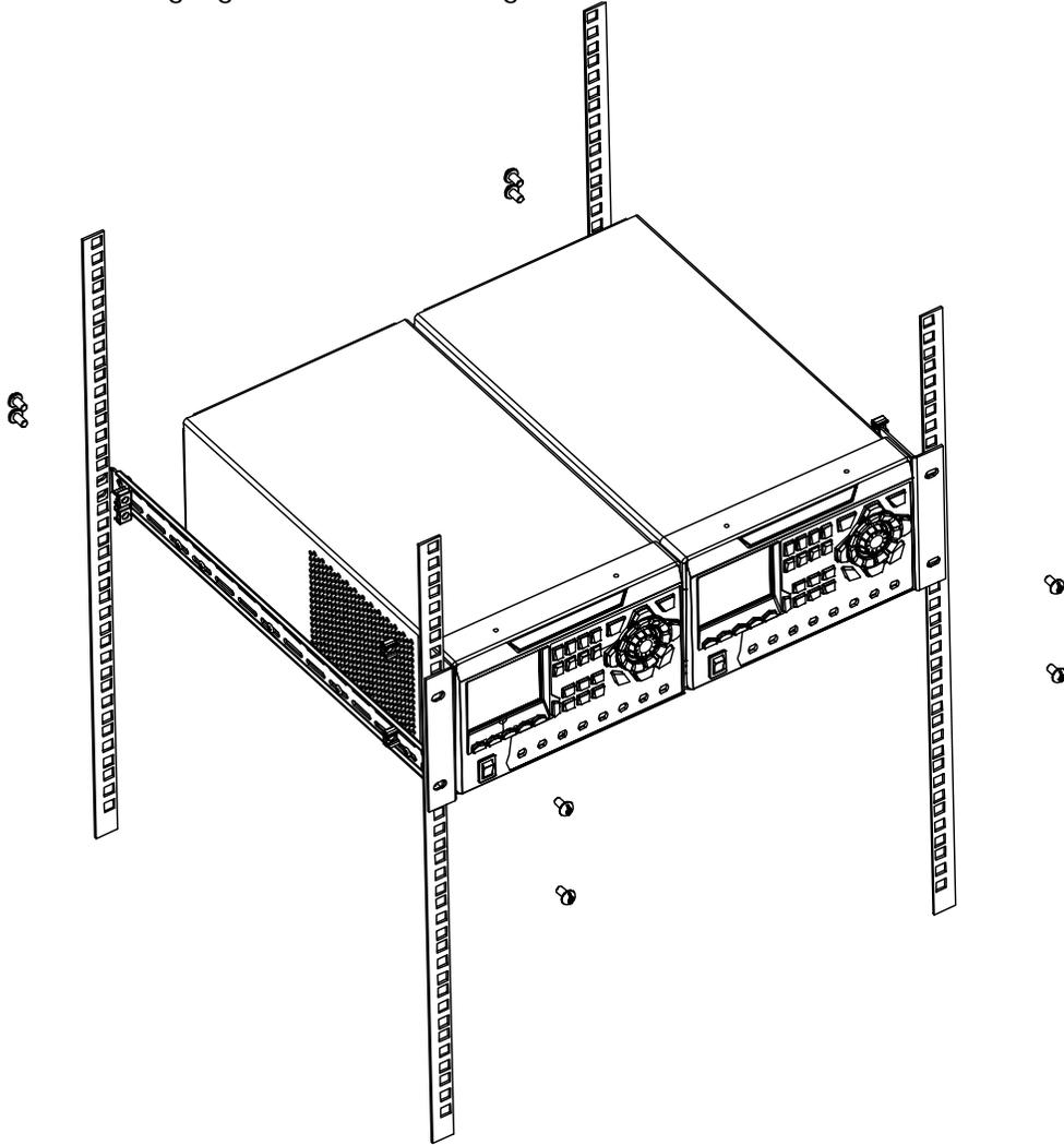
9. The rack-mounted instruments are as shown in the figure below.
