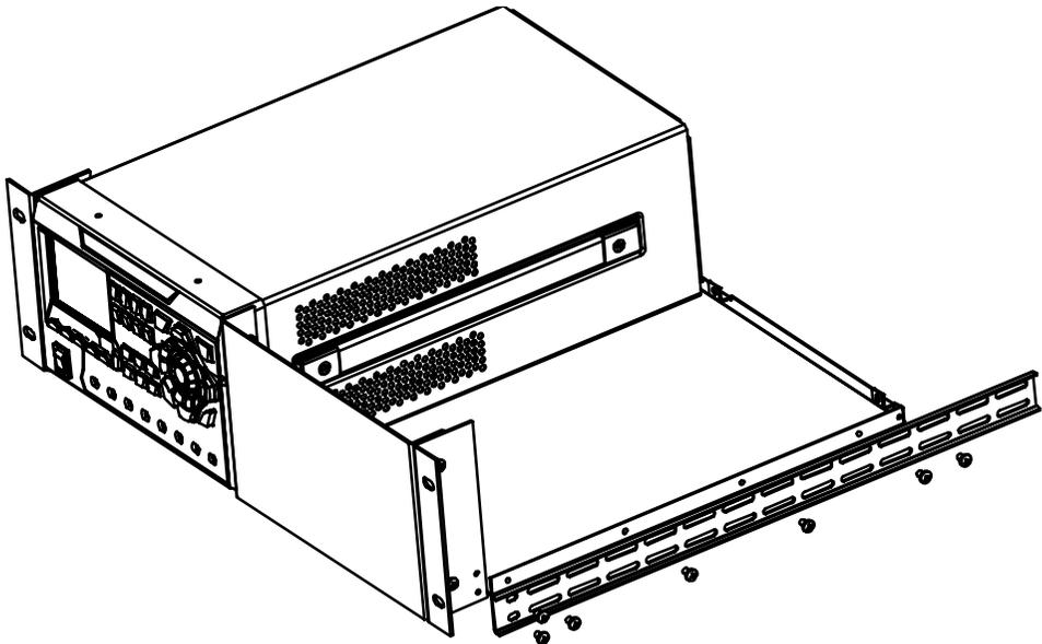
7. Fix the other rack rail at the left side of the rack support shelf using seven M4 screws.
