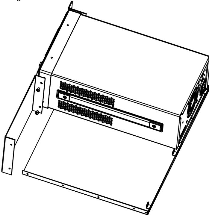
5. Fix the right fixing part to the right side of the front filler panel using two M4 screws.
