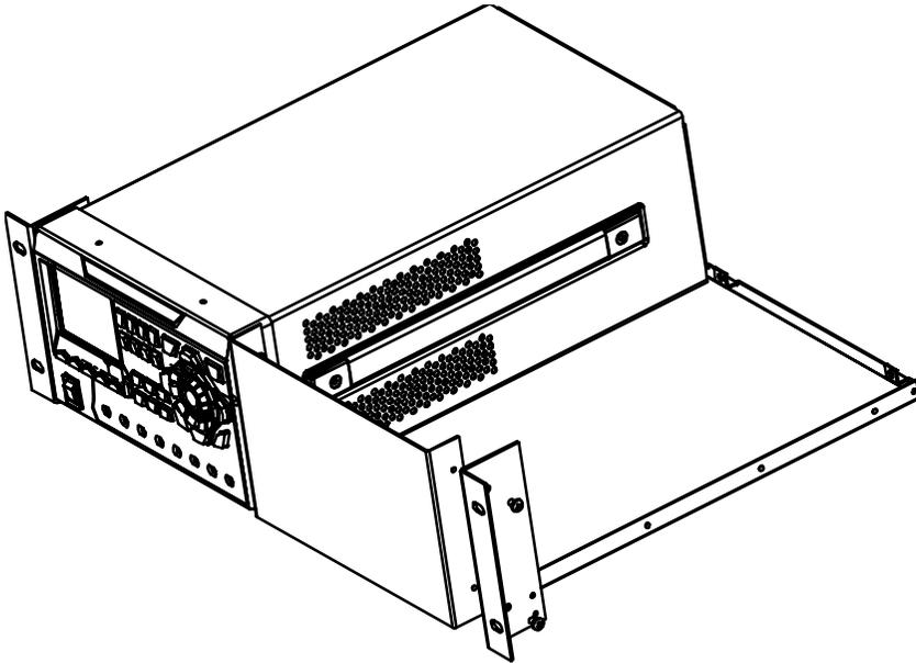
6. Fix a rack rail at the right side of the rack support shelf using seven M4 screws.
