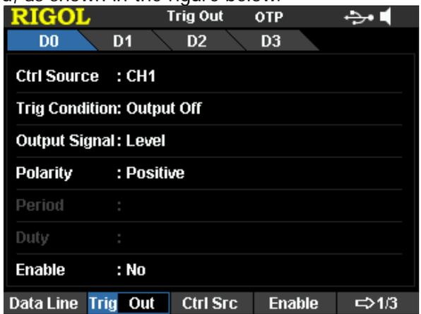
Figure 2-7 Trigger Output Setting Interface
