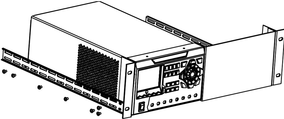
8. Fix the two side beam fixing parts to the end parts of the left and right rack rails respectively using four M4 screws.
