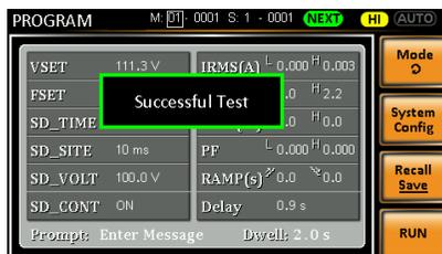
P/F: If one of the test results is judged a fail, then FAIL is displayed on the screen.
