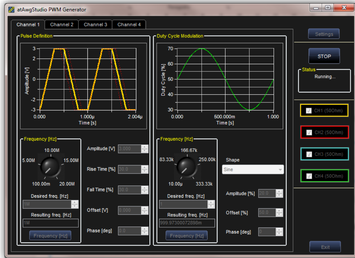
Figure 81: PWM Generator – Run state
