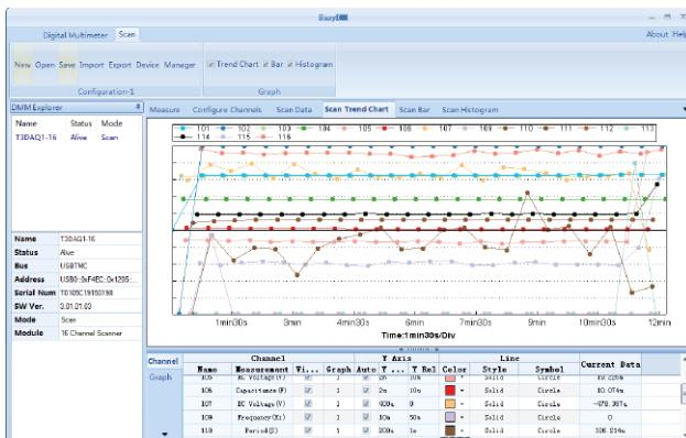
To view the scanned data visually, the software has Trend Chart, Histogram and Bar graph. All the graphs also has user customizable options such as colour, axis scales, type of curve etc.
