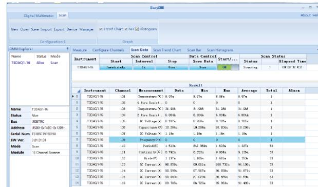
Different measurement settings such as Scan interval, Start and Stop time can be set from the Scan Data menu. The Result section provides the live measurement data along with min, max and average values. It also provides total number of scans and number of Alarm for every channel.
