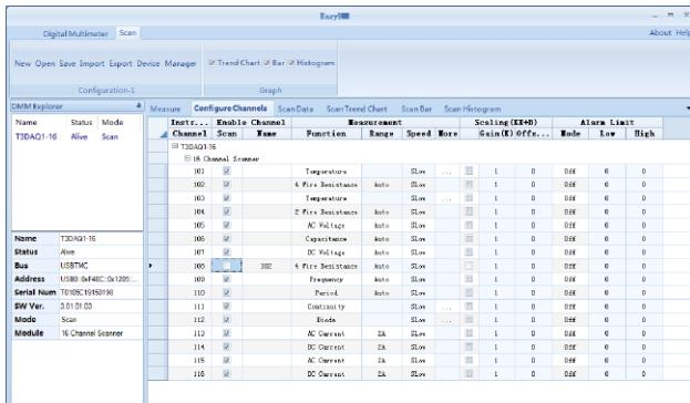
Configure Channels menu in the Scan mode can be used to enable channels as well as to configure various settings such as measurement function, range, speed of measurement. Channels can also be monitored within the defined limits by using Alarm Limit feature.
